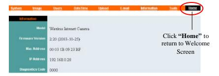
The Information table provides detailed information of the Wireless Internet Camera, such as the Model Name, Firmware Version, Mac Address, and IP Address.
